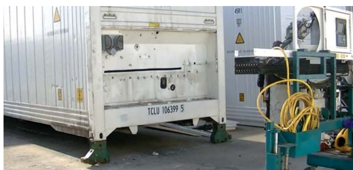
◀ Star Cool Integrated is a modular design, which also makes removal and re-fitting somewhat easier.
